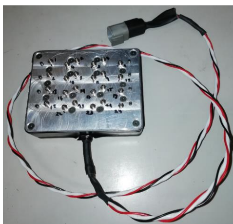
Figure 30 shows the completed pressure array ready to be installed on the vehicle.
