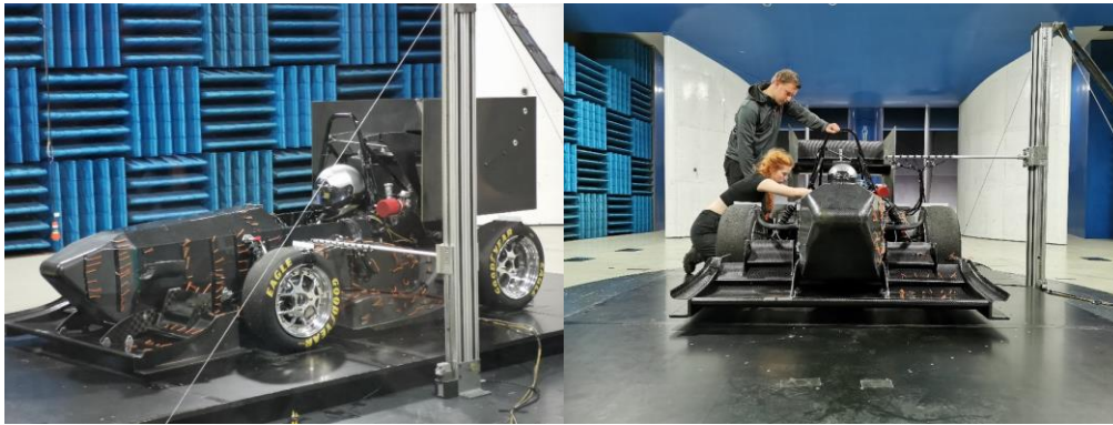
Figure 19 Shows the setup of the rake in the wind tunnel when the data was collected.
