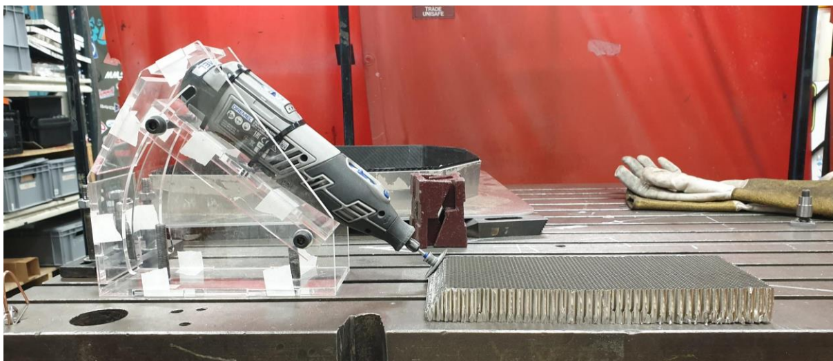
Figure 9.2: Prototype Dremel chamfering jig.
