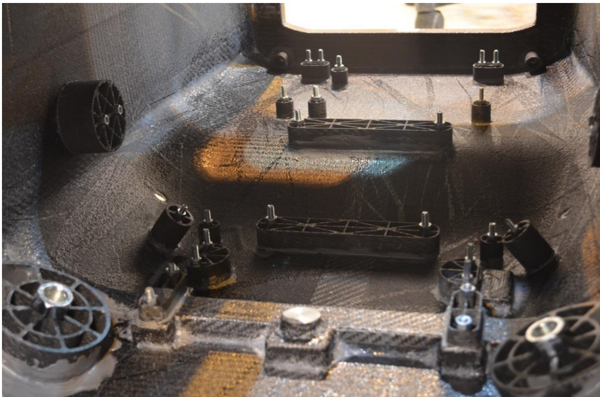
Figure 5.15: Placement of chassis inserts inside the mould, Revolve NTNU, 2014. [29]
