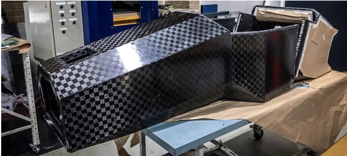
Figure 5.18: Two halves, front and rear, of the RMIT Electric Racing R19e monocoque. [30]
