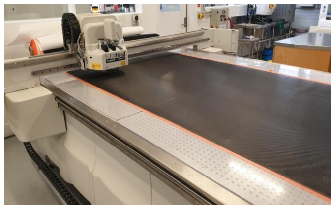
Figure 10.5: CNC ply cutting trial with Monash Food Innovation.
