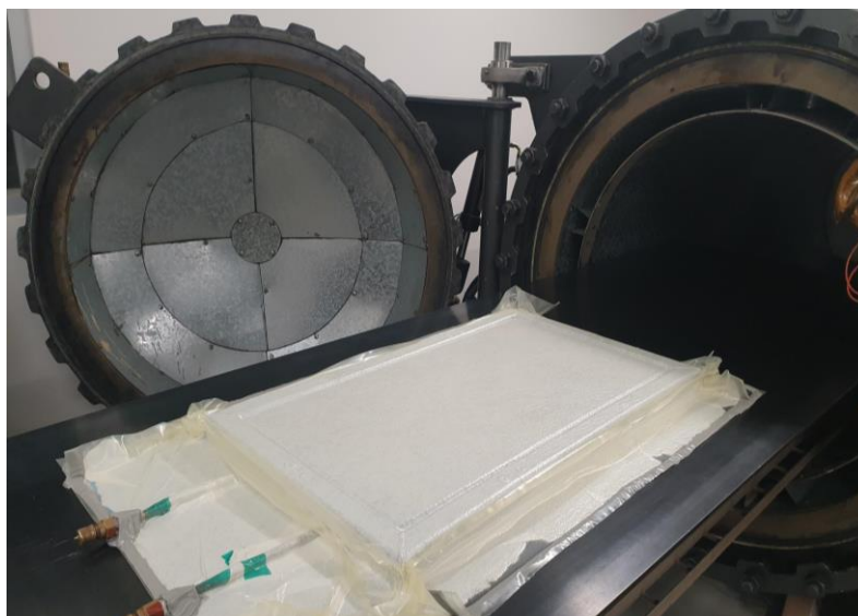
Figure 7.2: 3 point bend panel sample being loaded into the Monash University autoclave.
