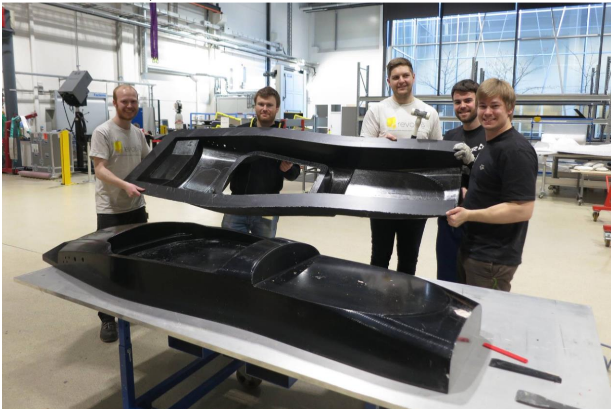
Figure 5.14: Monocoque plug and composite tool from Revolve NTNU, 2016. [28]
