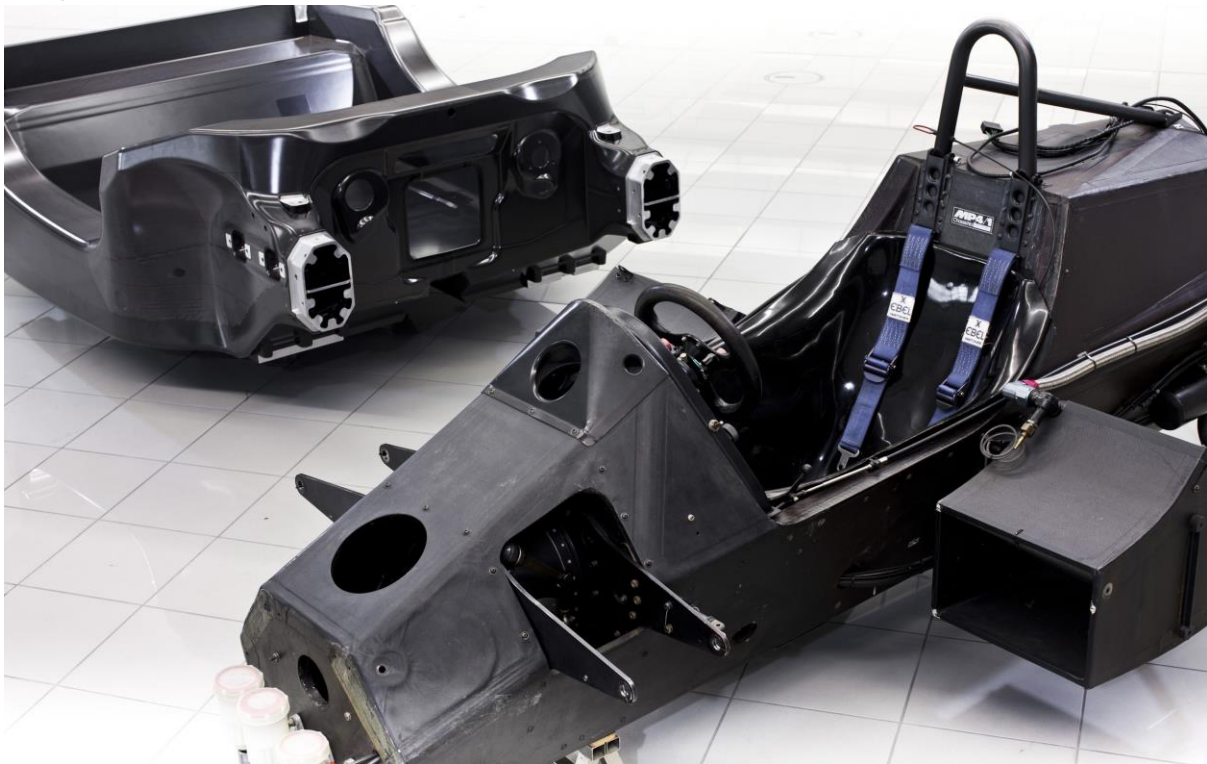
Figure 1.10: McLaren MP4-1 composite monocoque chassis (foreground) with McLaren MP4-12 road car monocoque (background). [10]
