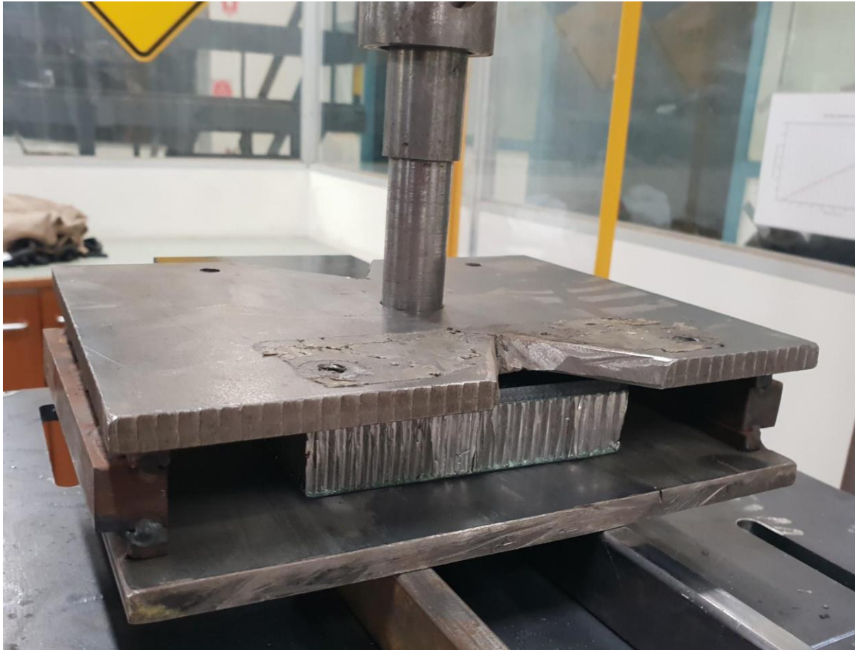
Figure 7.12: Perimeter shear test setup on the Instron UTM.
