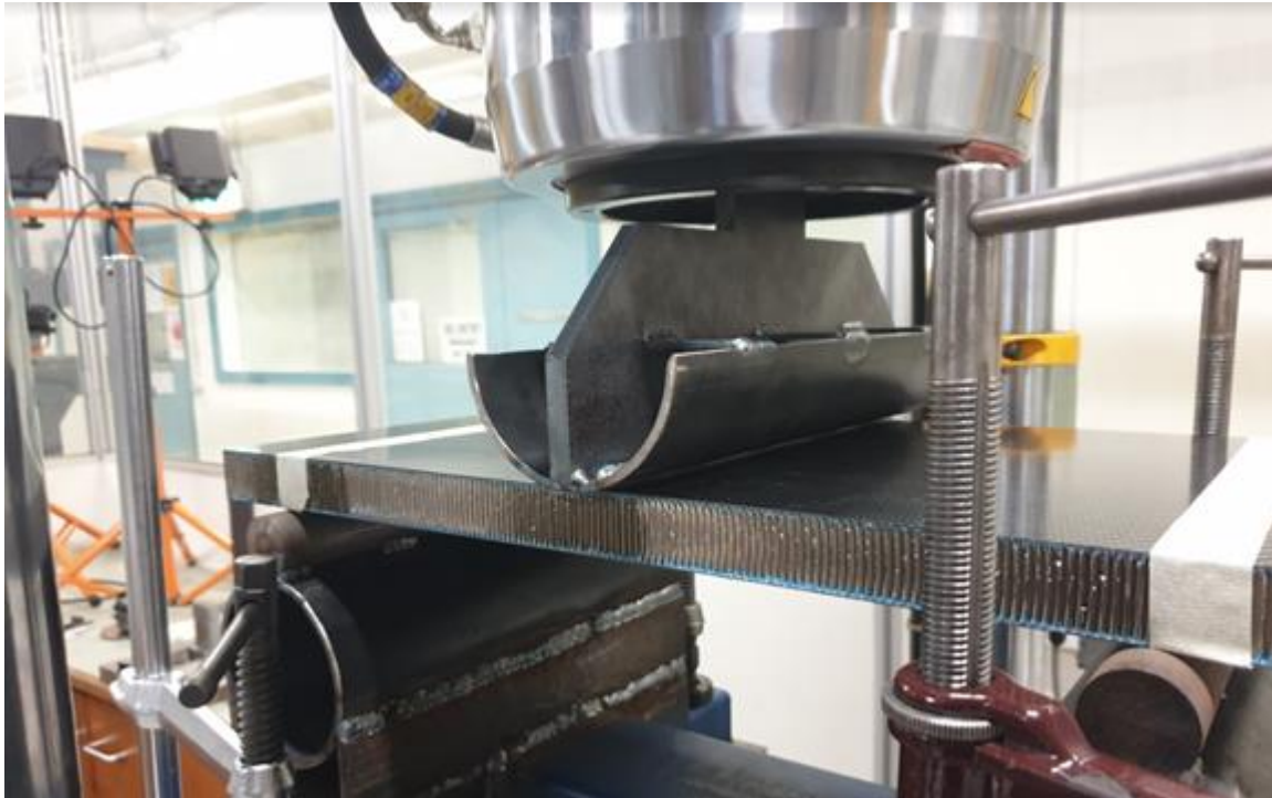
Figure 7.8: Composite panel specimen setup on the Instron UTM (note the modified panel supports).
