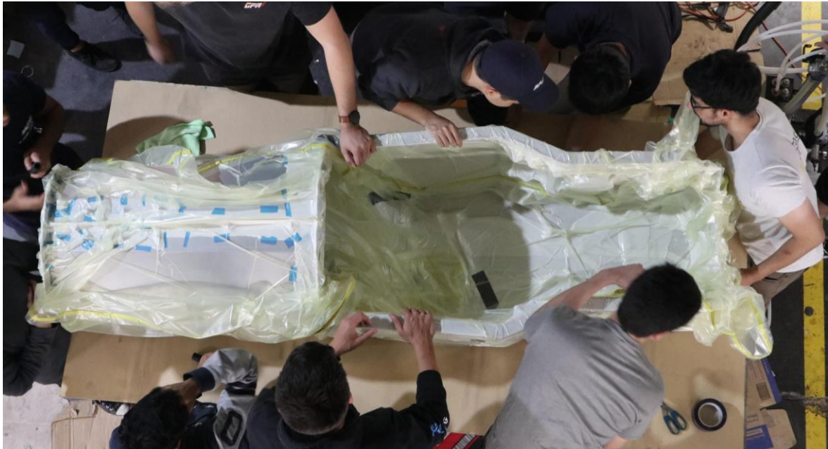
Figure 8.14: Vacuum bagging process for the mould.
