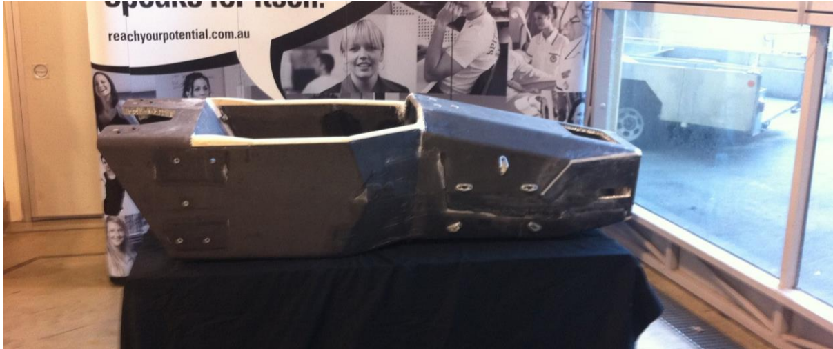
Figure 5.13: Edith Cowan University Racing 2014 cut and fold monocoque chassis. [27]
