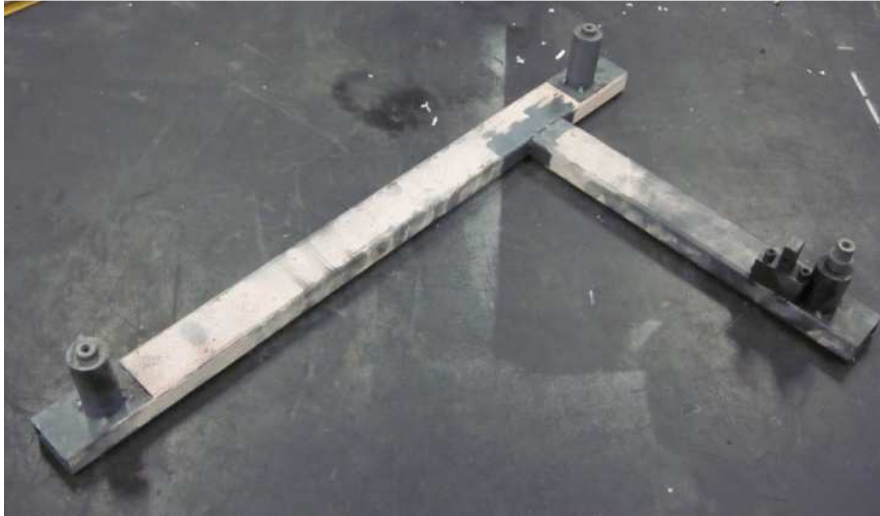
Figure 18: Simple rectangular hollow section fixture used for welding wishbones.
