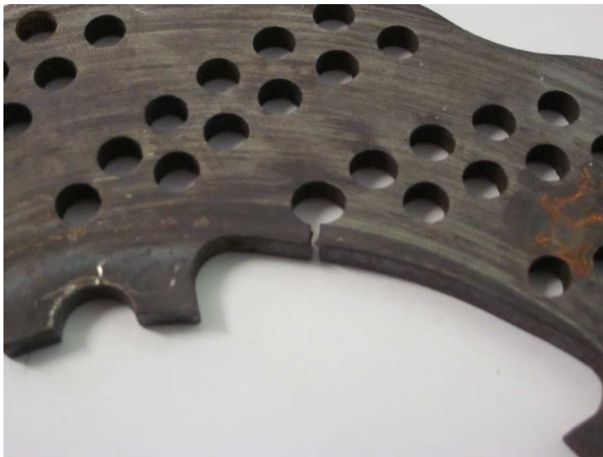
Figure 30: Failure due to cracking in a 2010 brake rotor. Several rotors failed this way.
