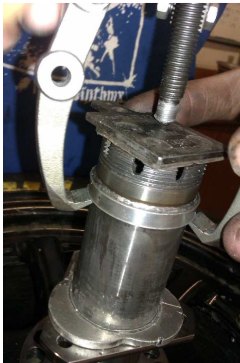
Figure 38: Crushed spacer being extracted from the front hub
