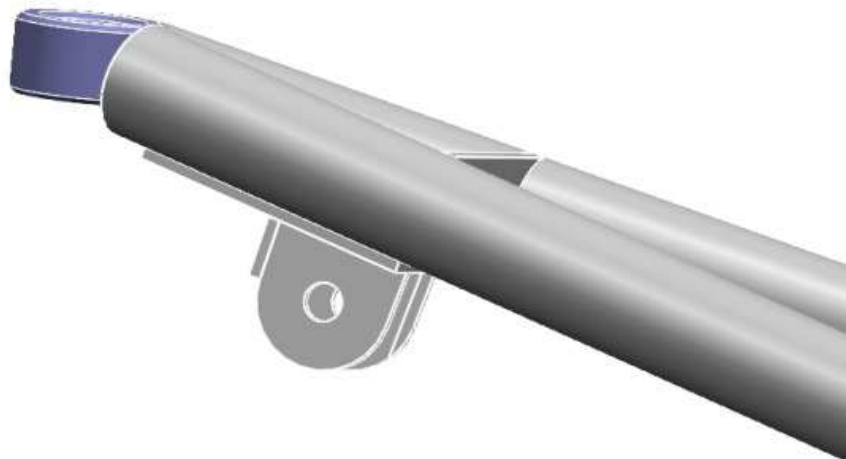
Figure 34: Inclined bearing cup arrangement on the front upper wishbone
