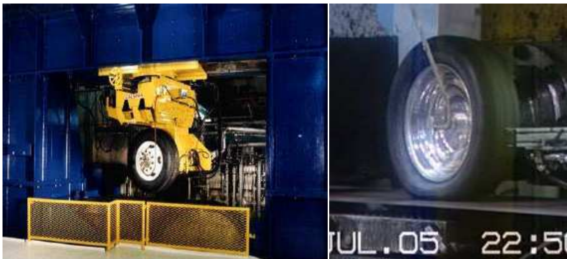
Figure 7, Calspan tyre test rig (left) and wheel being tested (right). Note the rotary union connected to control tyre pressure.
