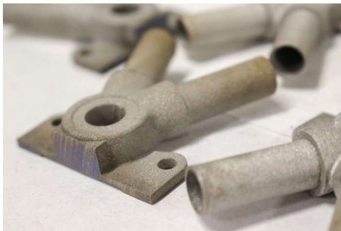
Figure 43 Front upper wishbone inserts and bearing cups printed by MCAM. The rough surface finish can be seen and provides a great adhesive bonding surface.
