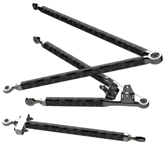
Figure 39 Rear right carbon fibre wishbones final CAD design and render.
