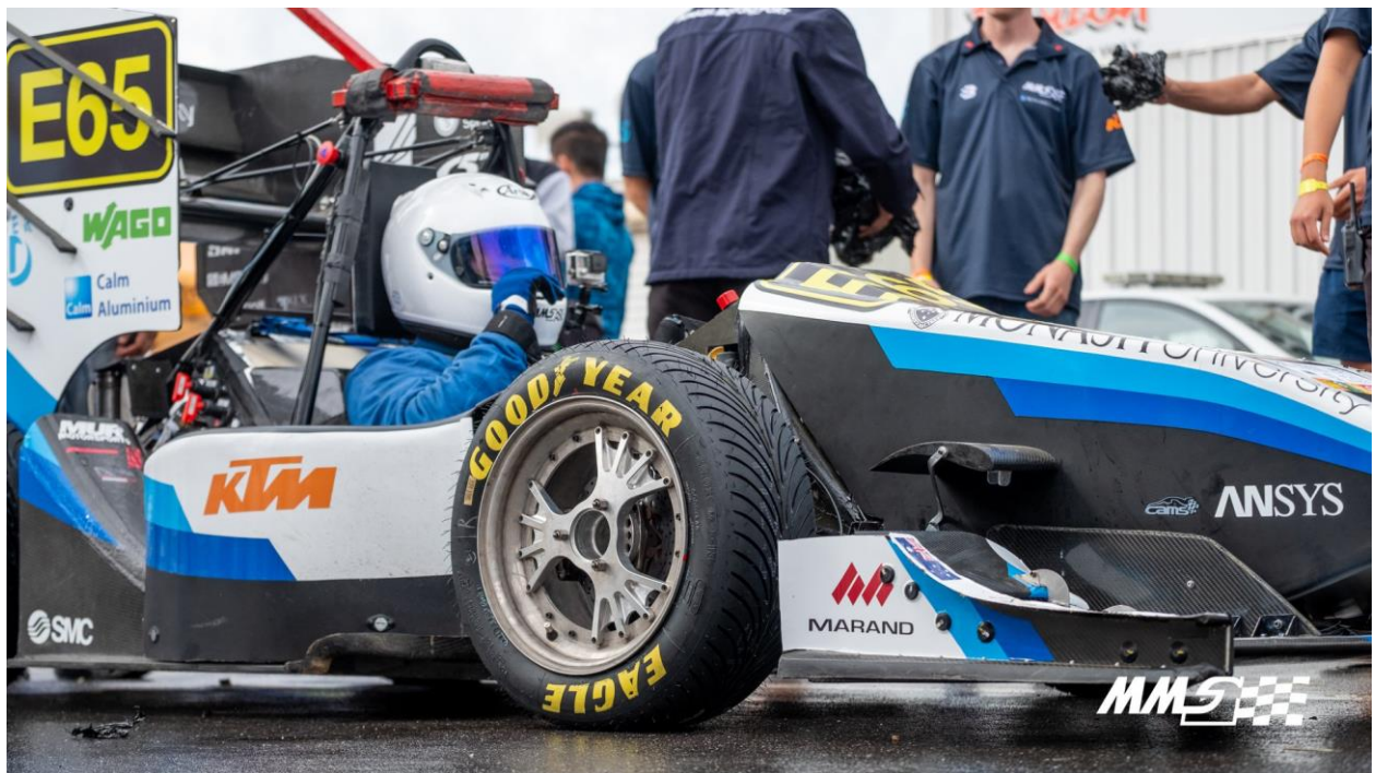
Figure 3 M18-E with a three-piece aluminium wheel supporting the 13-inch Goodyear wet tyre. The same concept will be used in 2019, with the dry Goodyear D2704 tyres and a redesigned wheel centre.
