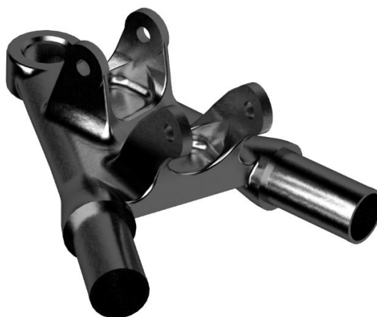
Figure 40 Rear lower titanium outboard design, CAD render.
