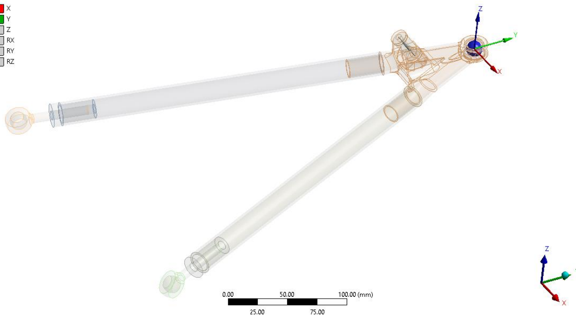
Figure 78 Fixed z-axis translation and fixed rotation at the outboard spherical bearing.
