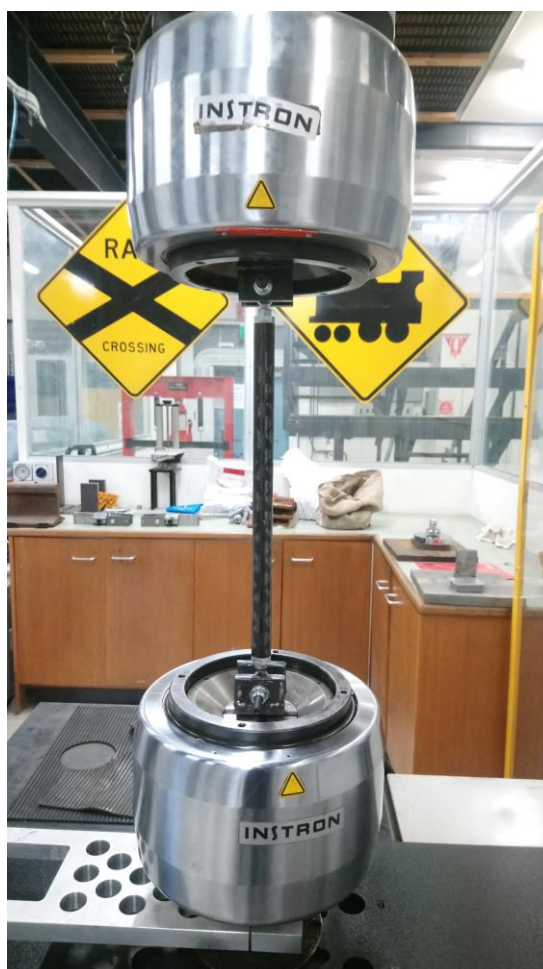
Figure 26 Buckling test performed on the Instron at 5 mm/min compression.
