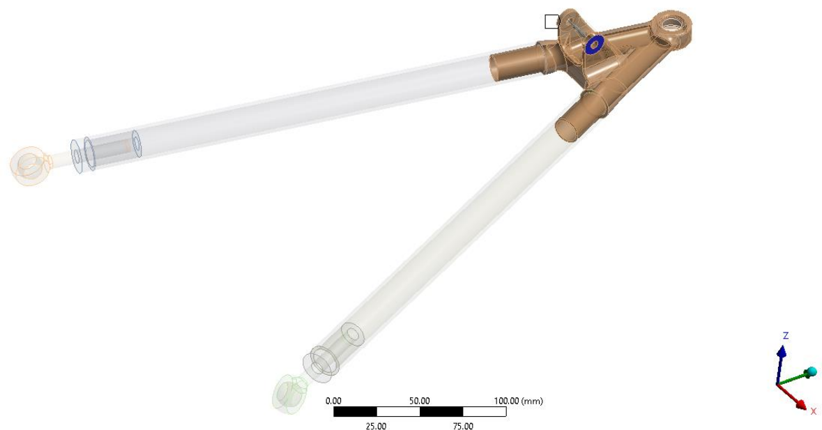
Figure 79 Longitudinal spring joint used to model the bolt clamping force of the shock clevis.
