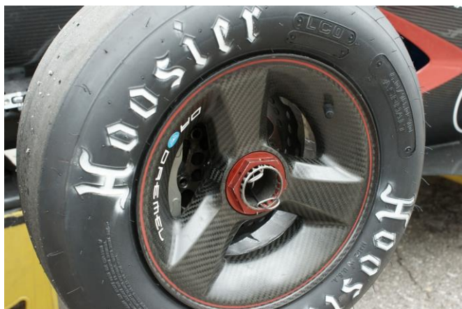
Figure 5 A one-piece carbon fibre wheel design by TU Graz Racing Team.
