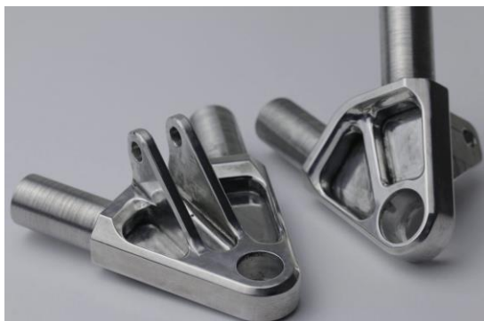
Figure 24 Machined aluminium inserts and bearing cups by NTNU Revolve.
