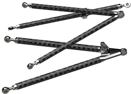
Figure 37 Front right carbon fibre wishbones final CAD design and render.
