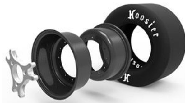
Figure 7 The 2017 Monash Motorsport three-piece wheel design, featuring carbon fibre wheel shells and an aluminium wheel centre.
