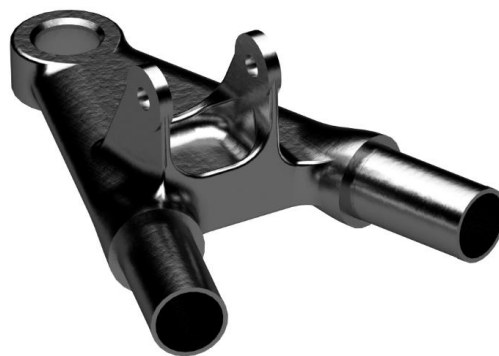
Figure 38 Front lower titanium outboard design, CAD render.
