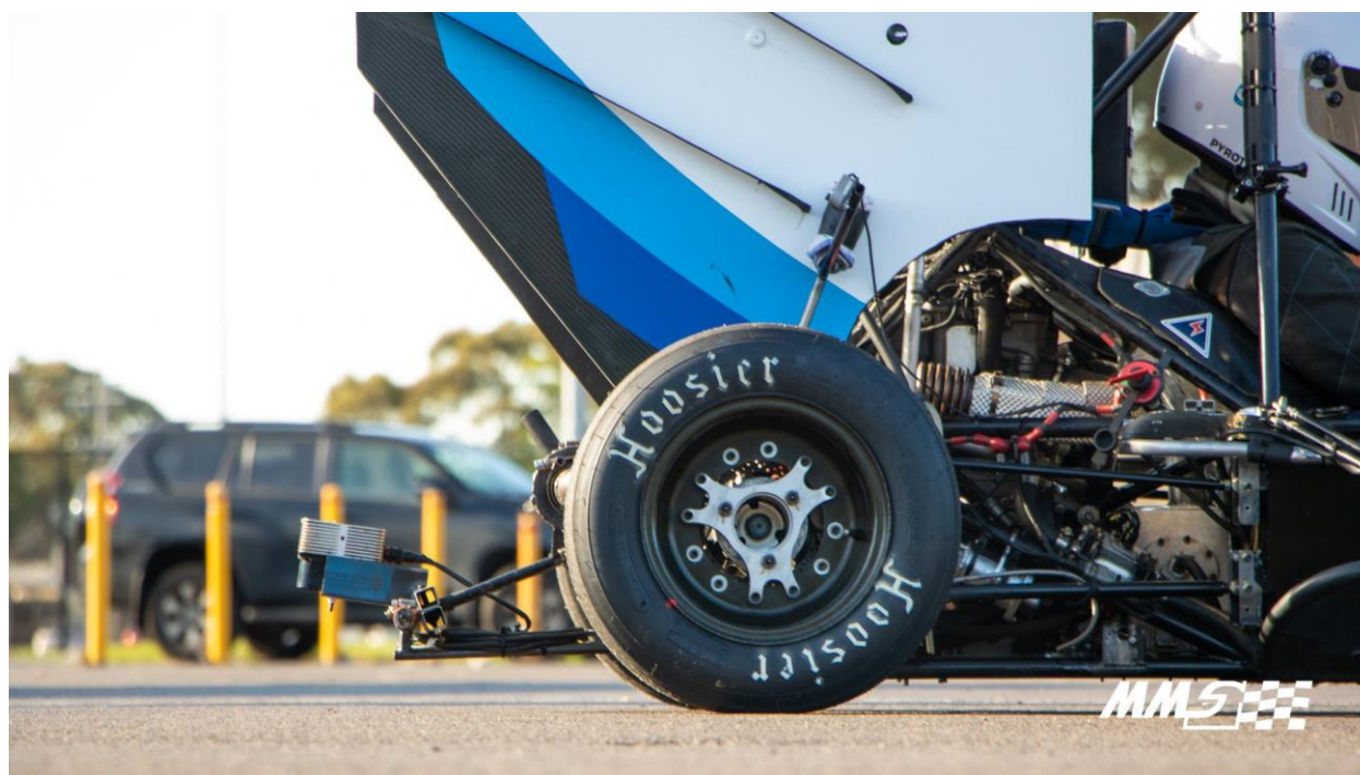
Figure 4 M18-C with the 10-inch Hoosier tyres and carbon fibre wheel shells, first manufactured in 2015.
