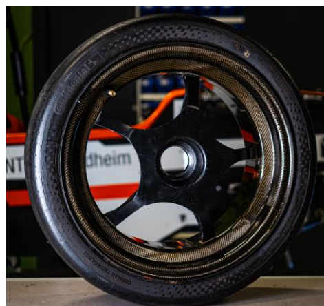
Figure 6 A two-piece wheel design by Revolve NTNU.
