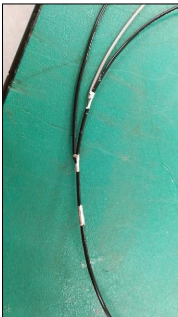
Figure 5.12: Splicing using Mechanical Crimps
