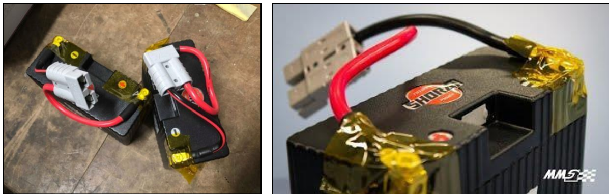
Figure 5.45: Shorai Battery Leads Manufactured and Installed
