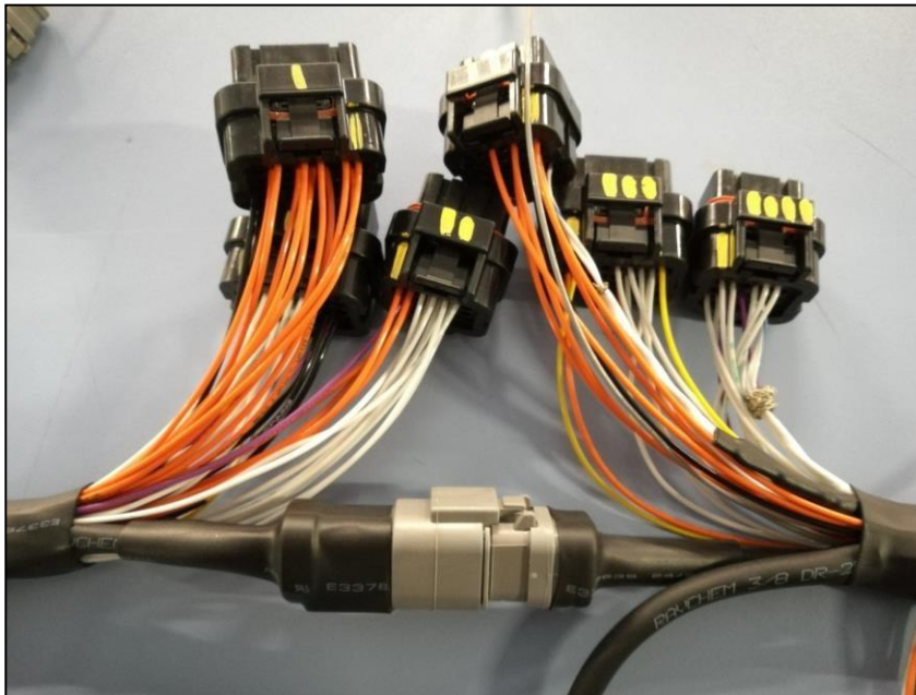
Figure 5.23: Superseal Connector Pinning Process
