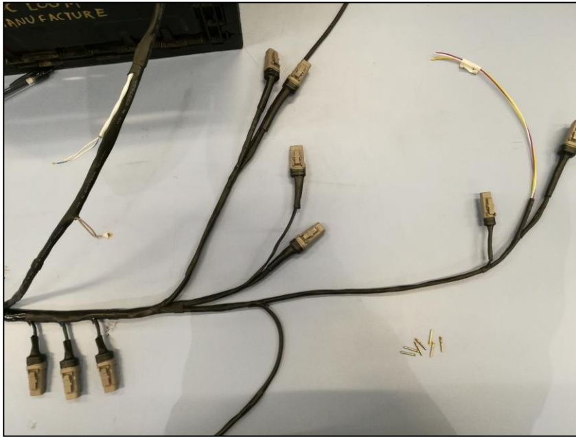
Figure 5.22: DTM Connector Pinning Process
