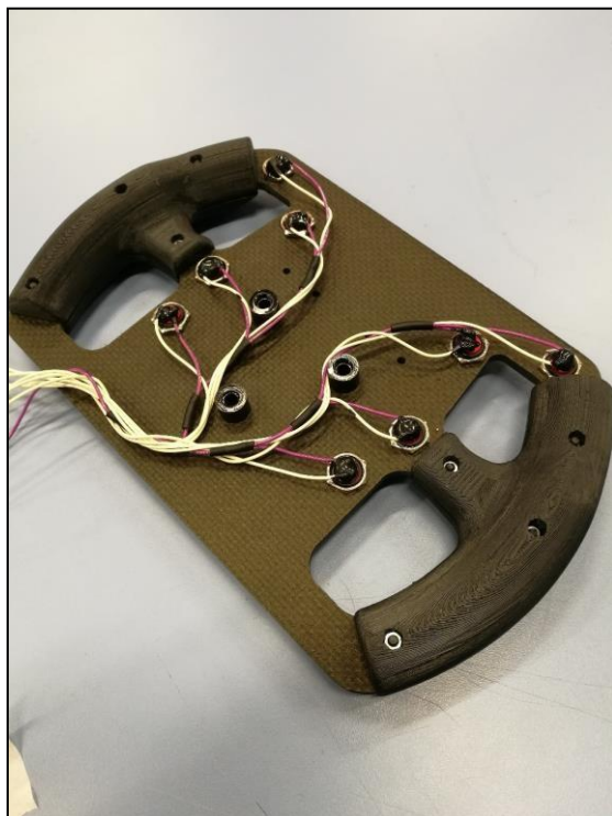
Figure 5.47: Epoxy on Buttons, Grounds Spliced, and Wires Routed
