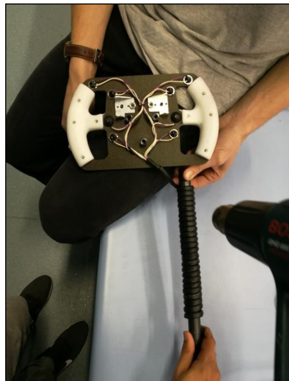
Figure 5.48: Tightly Twisting Around Metal Bar While Heating
