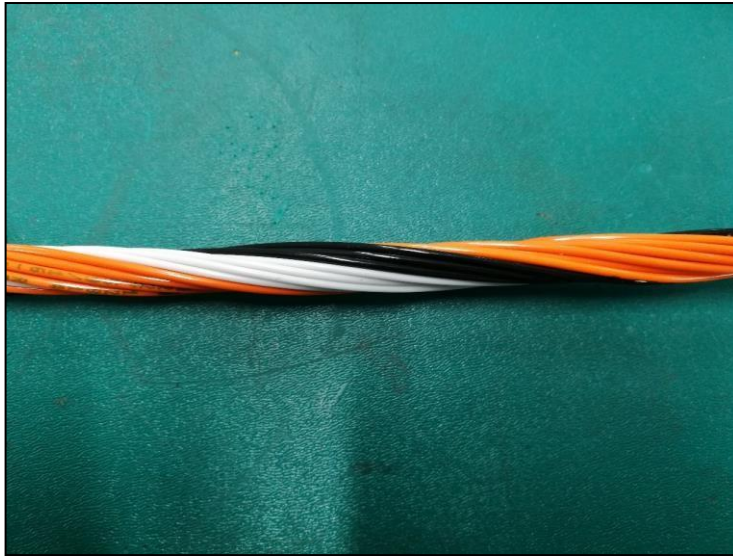
Figure 5.14 (left) & Figure 5.15 (right): Concentric Twisting
