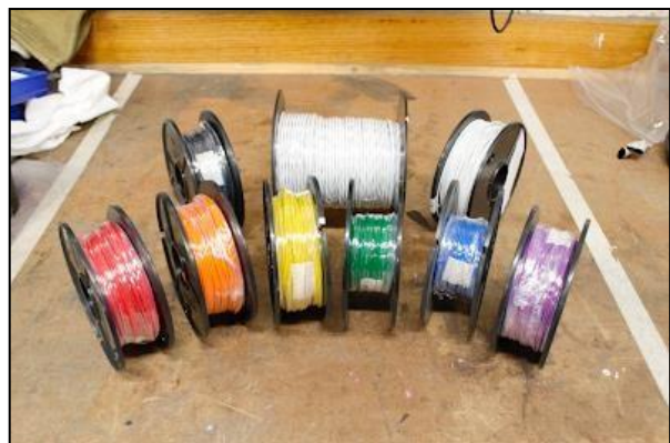
Figure 5.4: 20/22 AWG Single and Multi-Core Tefzel Wire
