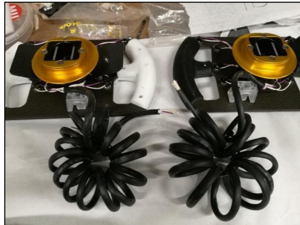
Figure 5.33: Cable Tie Mounts Being Glued to Steering Wheels
