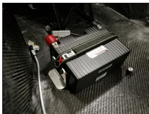
Figure 5.46: Battery Mounted in Final Position on Car
