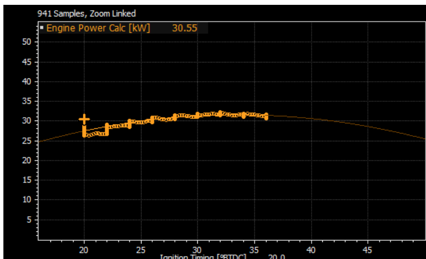
Figure 39: Ignition sweep at 8500rpm, 70 kPa MAP
