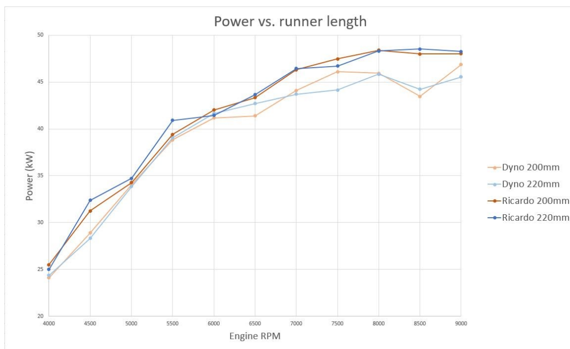
Figure 13: Power vs engine speed for 200 and 220mm runner lengths
