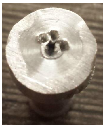
Figure 32: Argon restrictor plug with <1mm hole.
