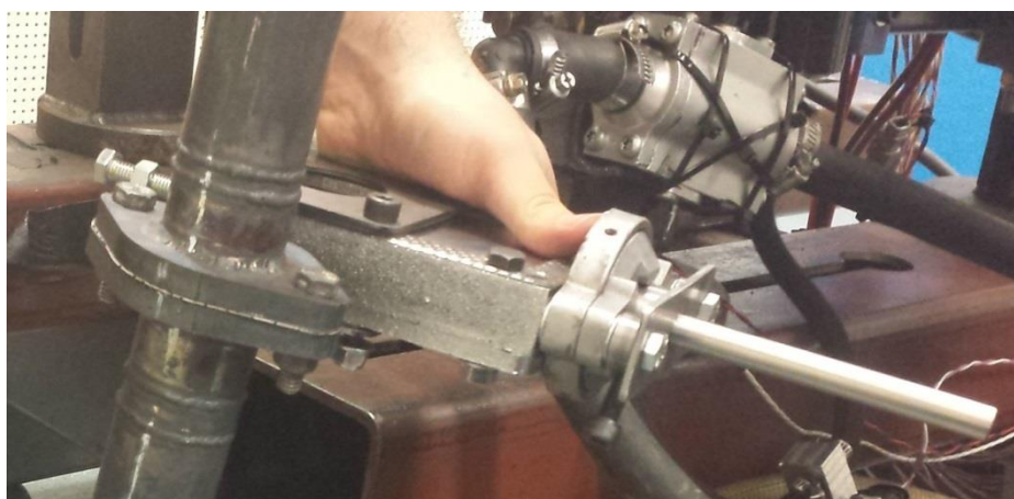
Figure 78: The exhaust brake prior to installation.
