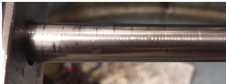
Figure 81: Marks made in the rod of the guillotine valve every millimeter which allow the valve to be opened to specific positions.
