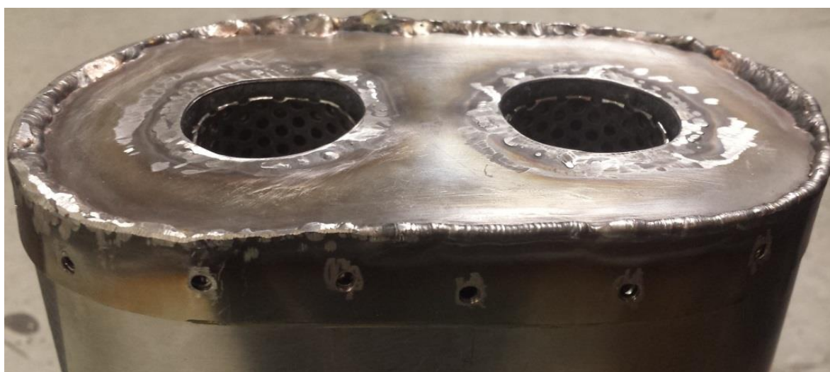
Figure 48: Welded and drilled stainless steel endcap. Note the rivet holes are not in line due to difficulties with the center punch and drill combined with the surface hardness of the steel alloy.
