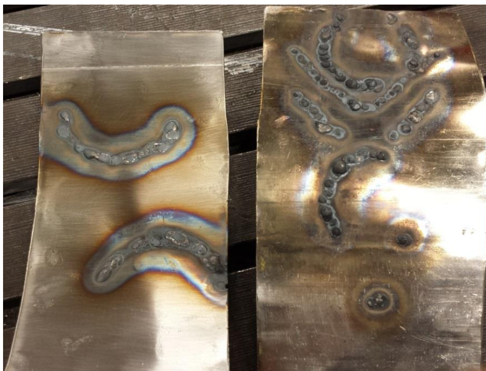
Figure 27: Left: Underside of purged weld. Right: Underside of unpurged weld. Note the difference in colouration and crystallisation.
