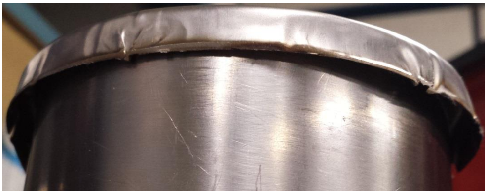
Figure 74: The highest quality stamped endcap out of the four attempts, placed over the stainless steel muffler main case to demonstrate the large gap and rippling which made the endcap unusable.
