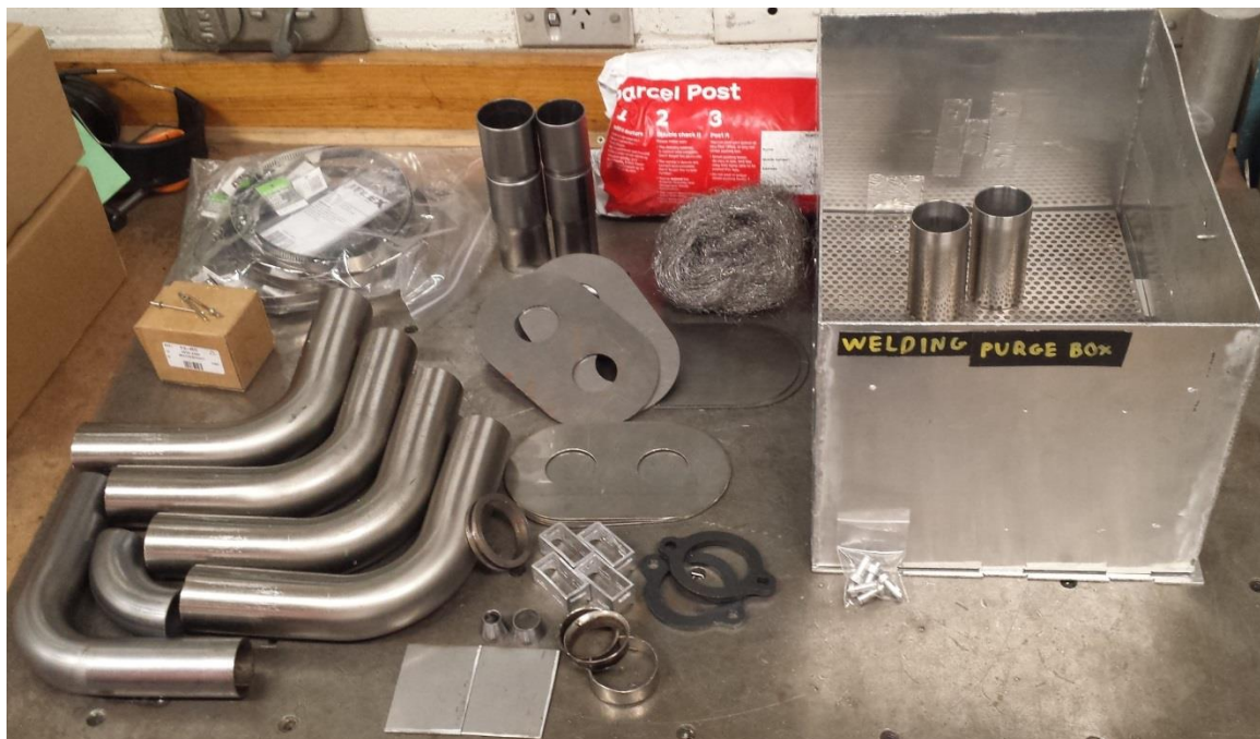
Figure f: Various parts used in the assembly of the exhaust, muffler and welding purge box.
