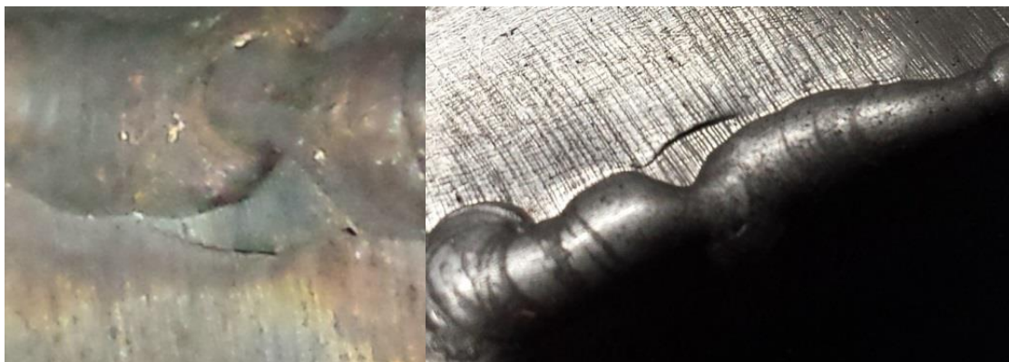
Figure c: Left: Small crack in a stainless steel muffler weld, main case to outer end bulkhead. Right: The same small crack after sanding the surface.
