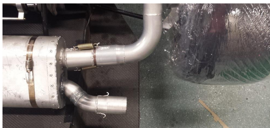
Figure 19: The mild steel muffler's side-facing outlet after further modification.
