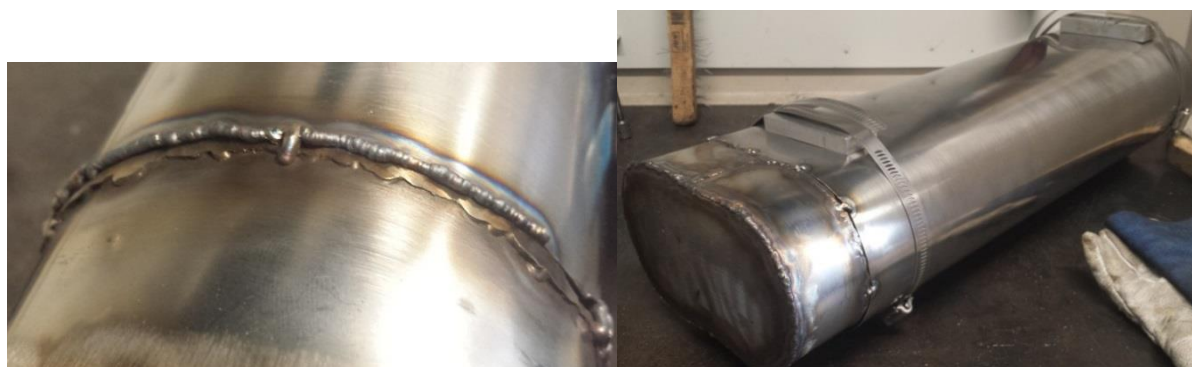
Figure 45: The end chamber tacked to the main case. Left: Close-up. Right: View showing hose clamp jigs.
