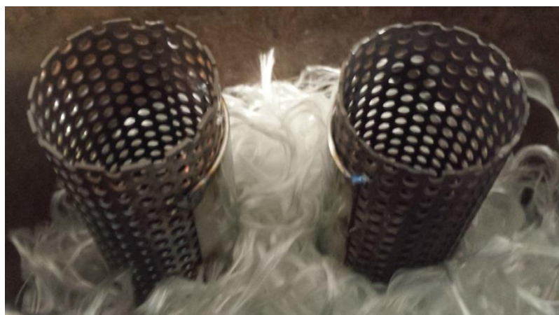
Figure 68: Repacking the stainless steel muffler with steel “shields” welded to perforated tubes.
