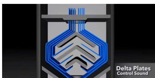
Figure 12: “Delta Plate” technology in a FlowMaster muffler (Kimbrough, 2014), showing how some noise (blue lines) are directed into channels between the plates.
