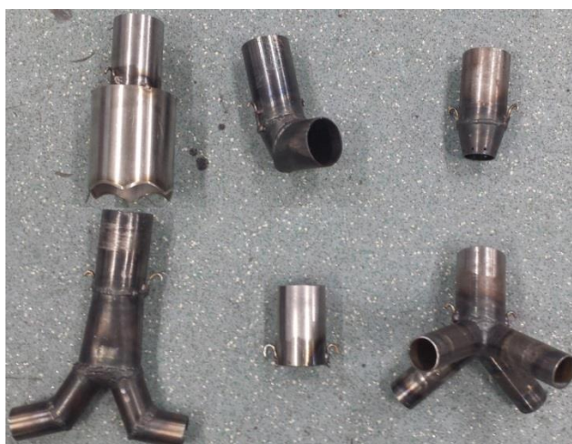
Figure 51: Outlet tips for testing. From top left: Sheathed, 90°, 1 inch, 1 inch twin, 1.5 inch, 1 inch quad.
