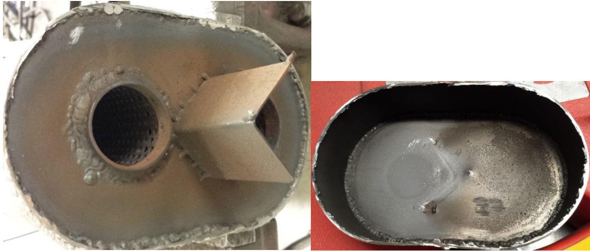
Figure 59: Left: Mild steel muffler inner bulkhead after removal of end chamber case. Note there is only one attached reflector plate. Right: The removed end chamber case.
