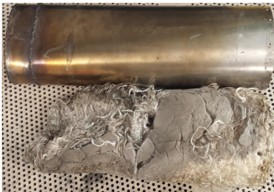
Figure 65: All the fibreglass absorptive material removed from the stainless steel muffler after 290km of testing. The fibreglass mass is lined up with the muffler case. Note the large missing mass of fibreglass to the left, on the closed end of the muffler.
