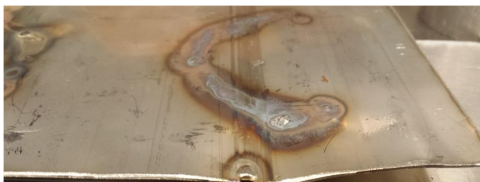
Figure 30: Underside of unpurged, clamped weld.
