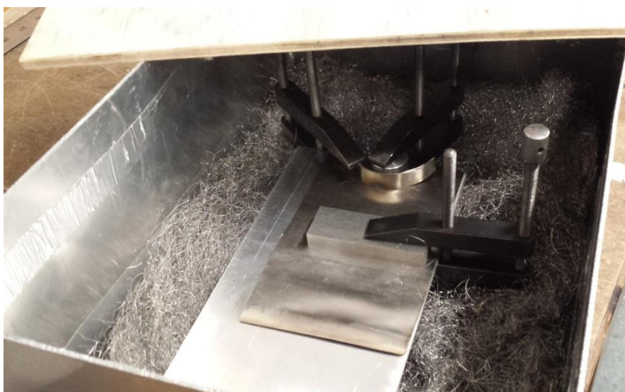
Figure 26: A stainless steel fillet weld jigged onto an aluminium sheet, inside the purge tank.
