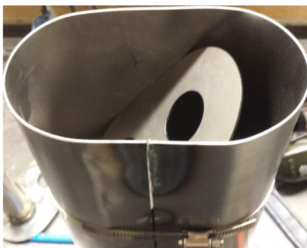
Figure 15: Spare bulkhead and hose clamp being used to shape/jig muffler case prior to welding.
