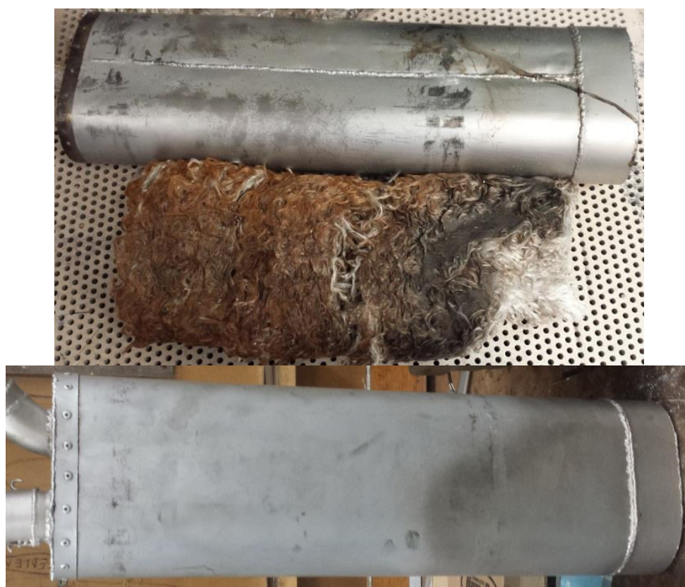
Figure 67: Top: fibreglass removed from the mild steel muffler, showing a missing mass in the bottom right. Bottom: The corresponding pattern of cured paint, in the same location as the hollow cavity.
