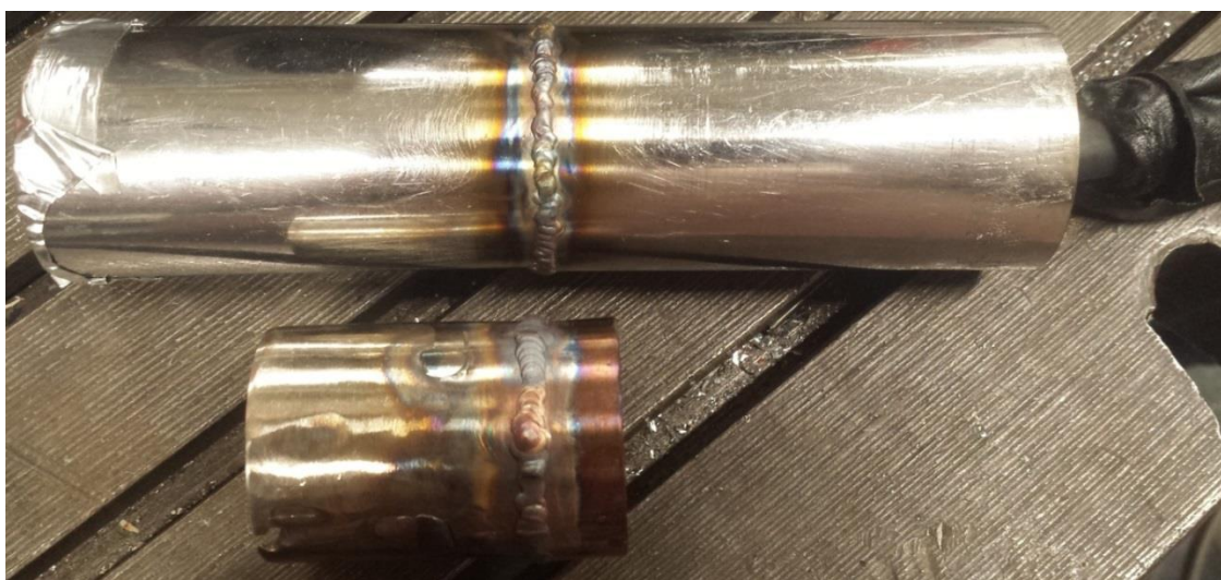
Figure 35: Outside of the purged (top) and unpurged (bottom) tube welds.
