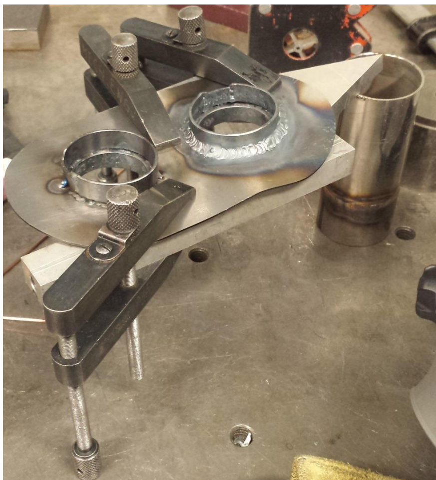
Figure g: Mild steel muffler inner bulkhead being welded using aluminium blocks and clamps.
