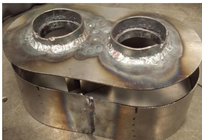
Figure 14: Mild steel end chamber assembly being inserted in the end chamber case prior to welding.
