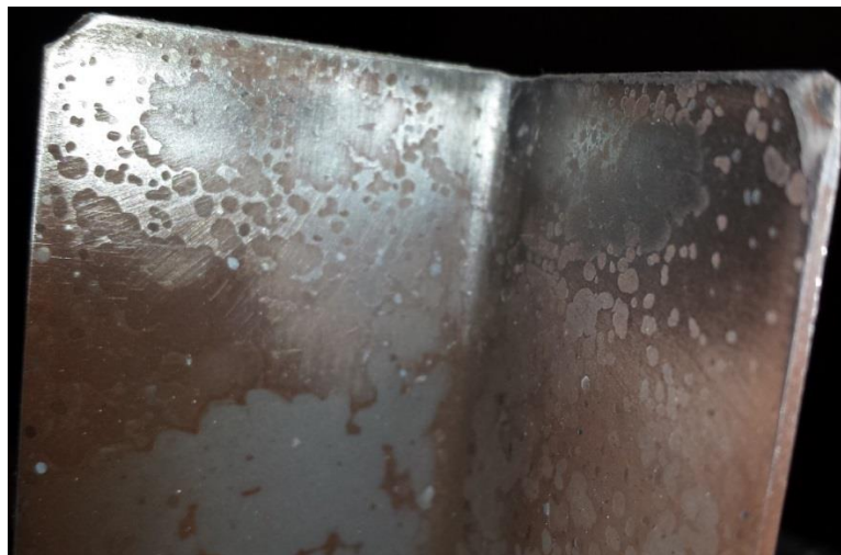
Figure 60: The failed reflector plate. Note the formation of highly reflective iron nitride, or "mill scale". This layer has high surface hardness and cannot be scratched with a file.
