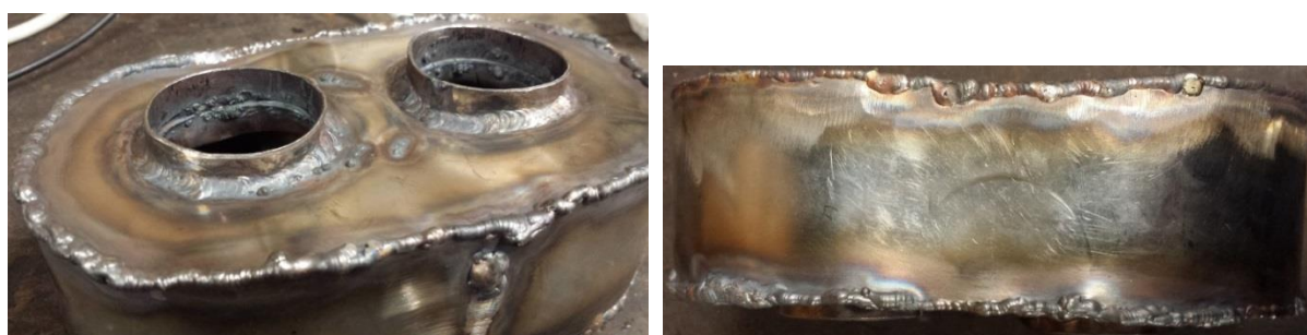
Figure 41: Welded and finished stainless steel end chamber. Left: isometric view. Right: Side view.
