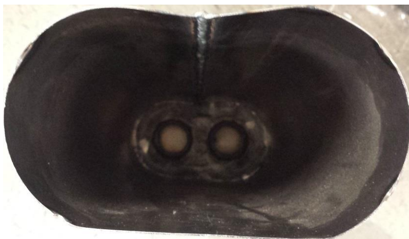
Figure 16: Mild steel muffler internal view prior to packing and endcap attachment.
