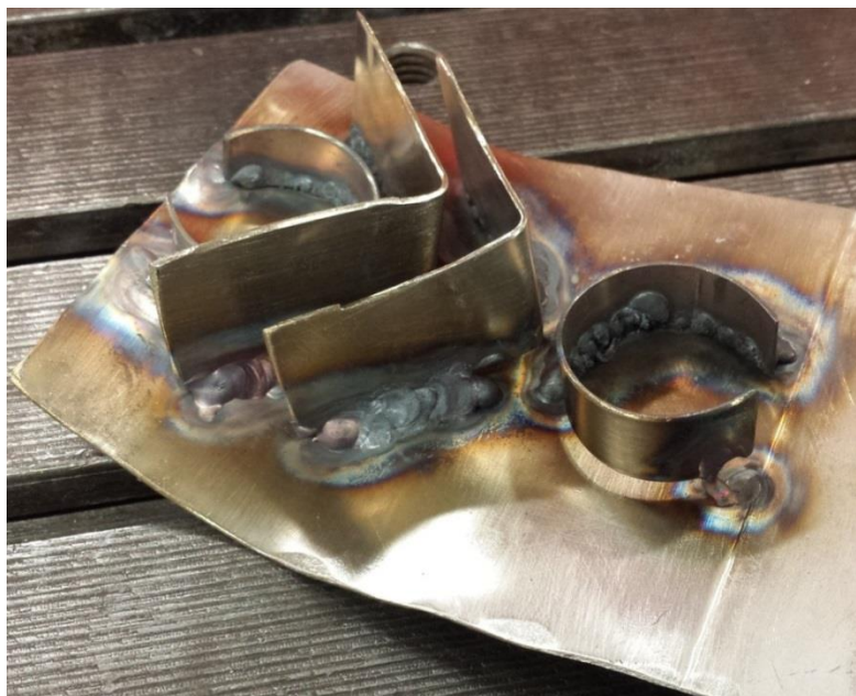
Figure 25: Resulting welds from unpurged control test in the purge tank. Note the excessive discolouration and warping, caused by the poor access conditions when welding over the walls of the tank.
