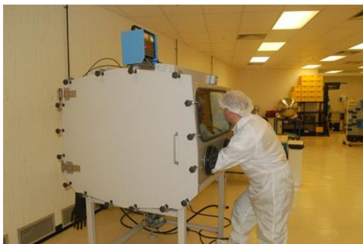
Figure 21: A technician operating a sealed welding chamber (RCW Aerospace Specialist Welding Solutions).
