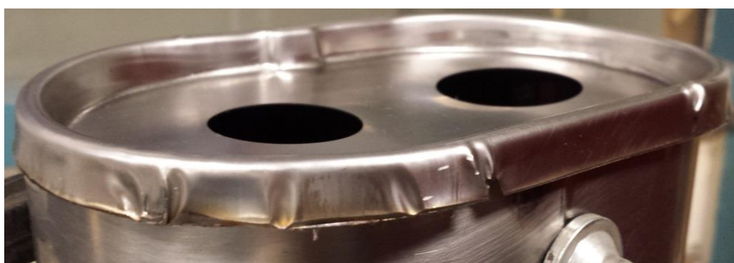
Figure 75: The same endcap as from figure 70, shown from above. The endcap is almost usable; a second iteration of the die would only need to solve the rippling problem.
