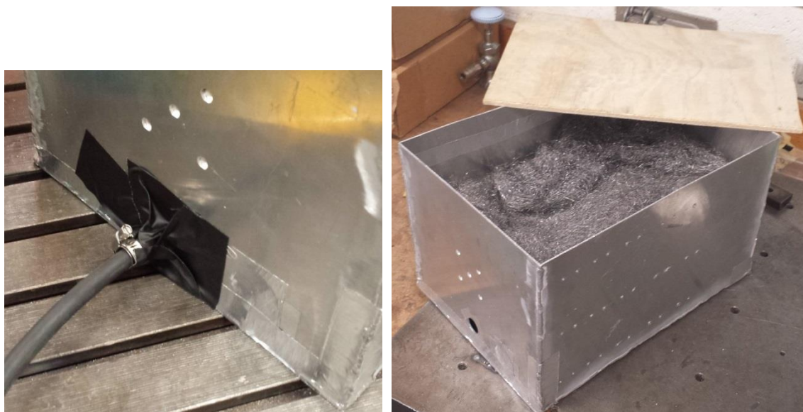
Figure 23: Left: Argon hose inserted into bottom section of tank. Right: Argon purge tank with lid open.
