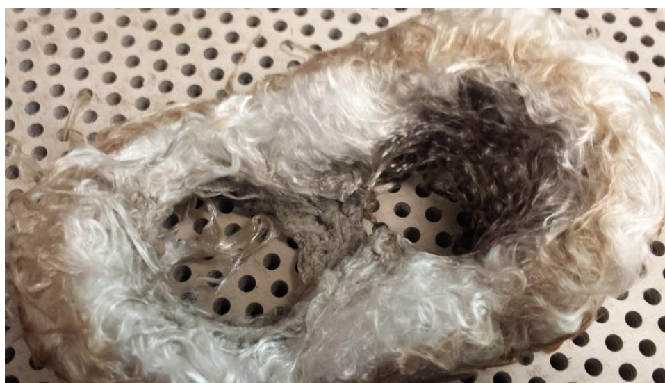
Figure 64: A cut-away of one of the holes formed between the perforated tubes.
