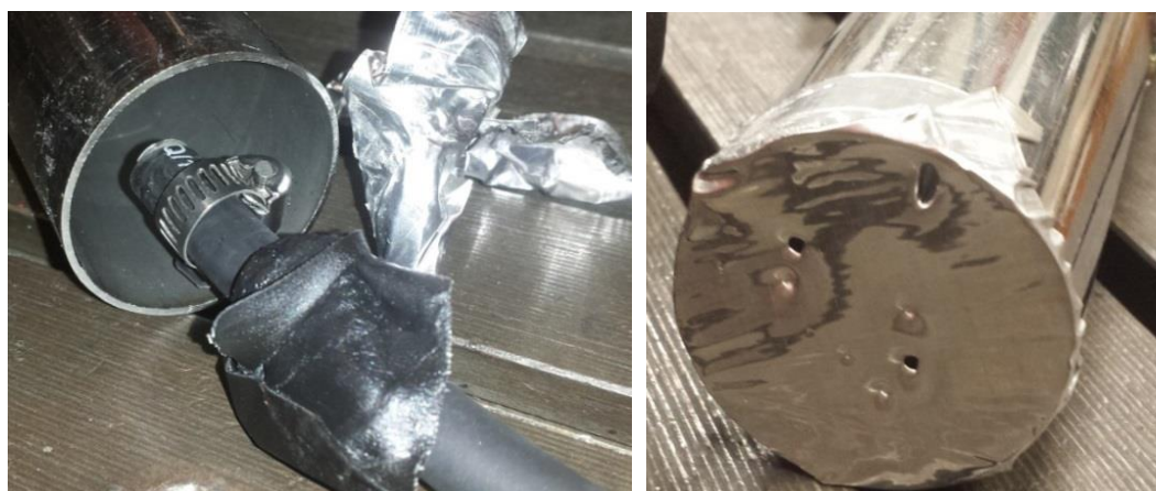
Figure 33: Left: Argon hose inserted in stainless steel tube, after removal of tape used to seal it. Right: Opposite end of the tube, showing punctured tape which prevents air from entering the tube.
