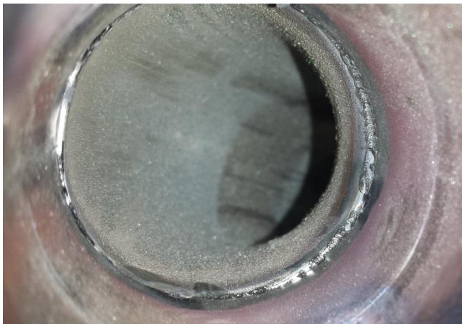
Figure 36: The inside of one of the manifold's welds. Note the lack of any crystallisation.
