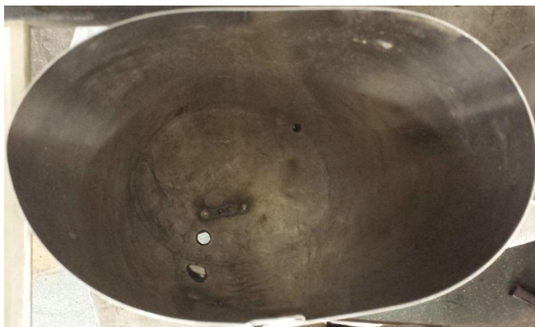
Figure 42: Top view of the stainless steel muffler case. Note the oblong shape and the lip at the bottom.
