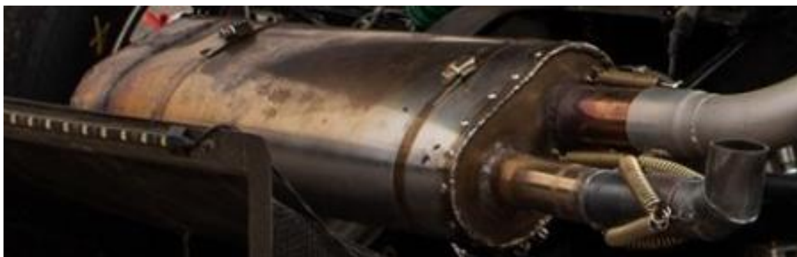
Figure 50: The stainless steel muffler installed on M20-C at FS Sydney 2020.
