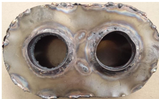
Figure 39: Partially welded stainless steel end chamber showing the intermittent style of weld seams.
