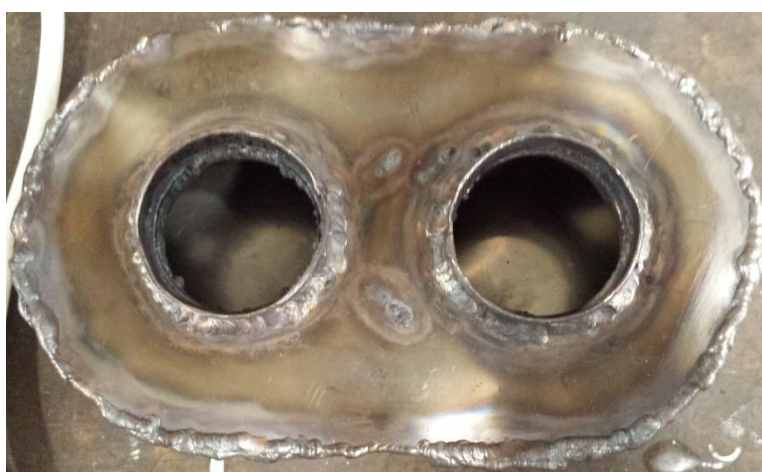
Figure 40: Welded and finished stainless steel end chamber, top view.
