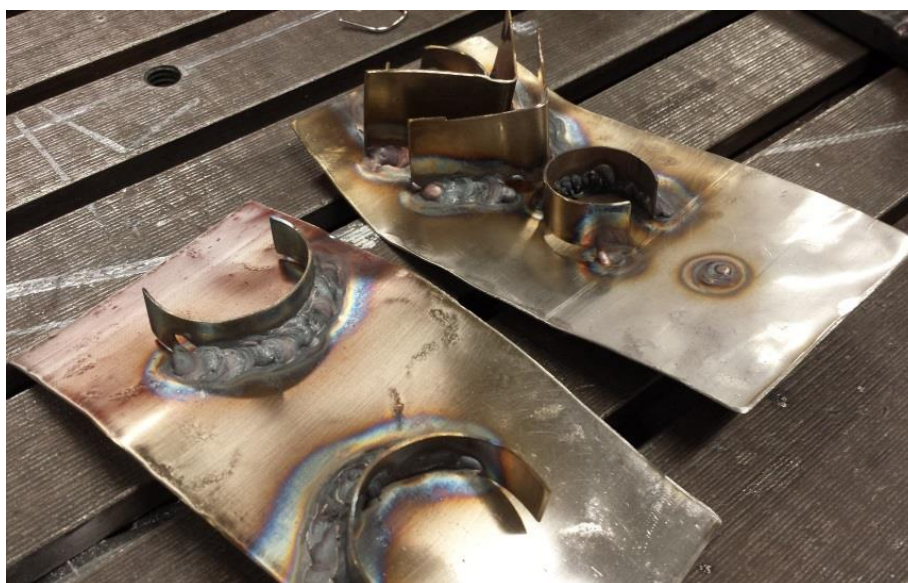
Figure 28: The two welded samples. Note the brighter colour of the purged sample in the foreground.
