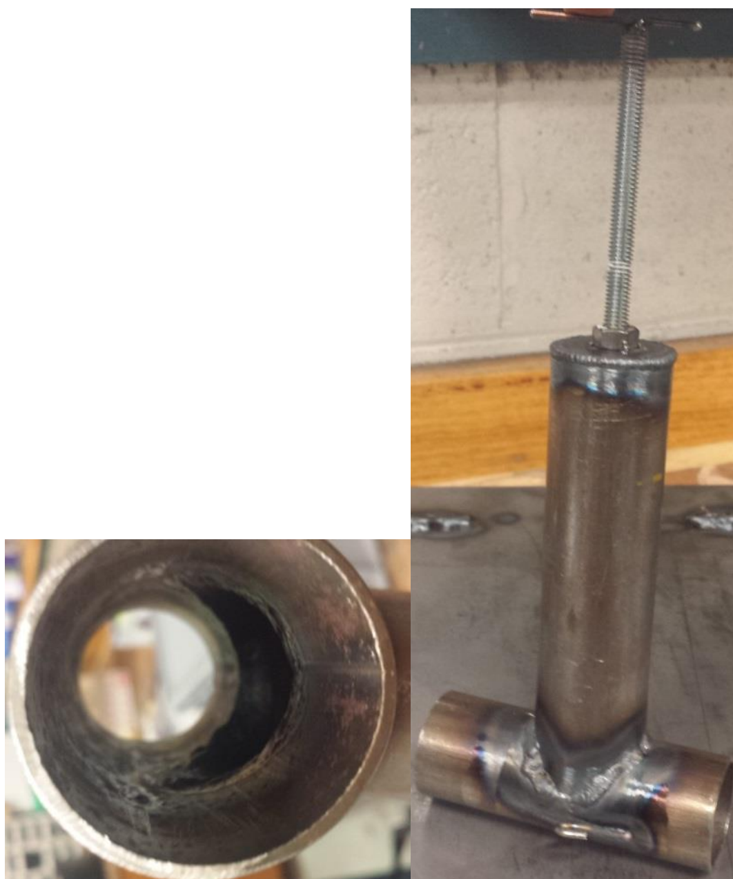
Figure 83: Left: View through the resonator's open section. Right: Photo of the resonator, showing the branched-off section and the threaded rod which allows for tuning.
