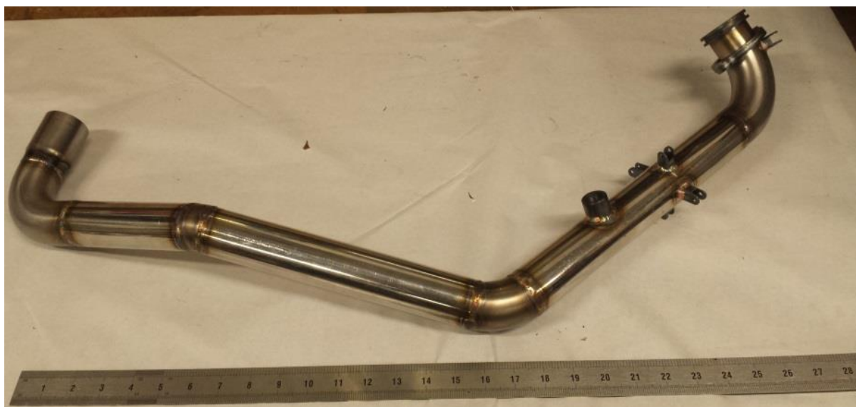
Figure 37: Fully welded stainless steel exhaust manifold for the M19-C and M20-C.
