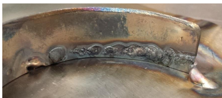
Figure 31: Back side of unpurged, clamped weld.
