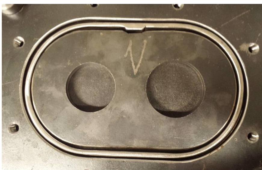
Figure 73: The combined die, showing how the male ring will fit into the female, pushing the flat endcap stencil into the cavity and forming an endcap shape.
