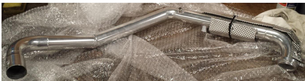
Figure 38: Stainless steel exhaust manifold after ceramic coating. The heat shield is mounted onto spacer prongs with a plastic cable tie in this photo, but it is swapped for a steel tie before installation on the car.
