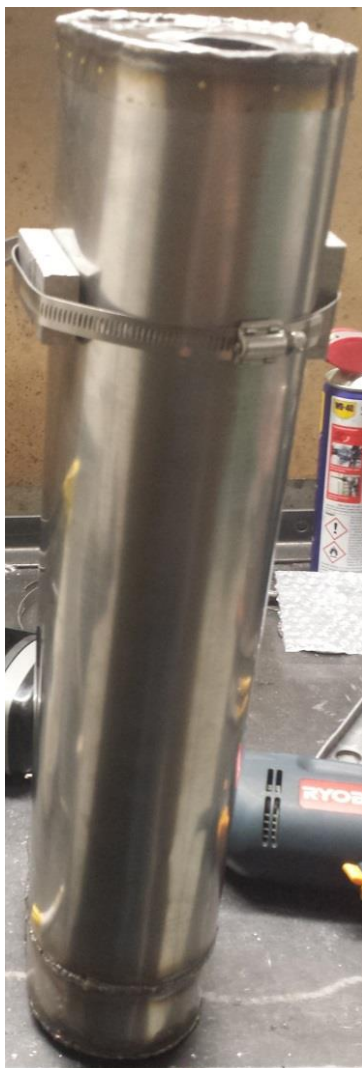
Figure 49: Stainless steel muffler assembled and standing on its end chamber. Note the significant longitudinal twist. This is likely caused by the welds, or a lack of constraining jigs during welding.
