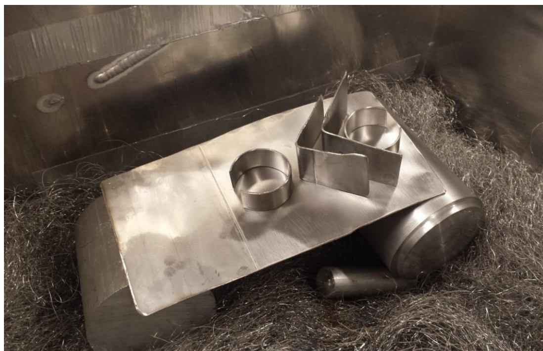
Figure 24: Stainless steel inner bulkhead mock-up resting on spare billets in the purge tank.
