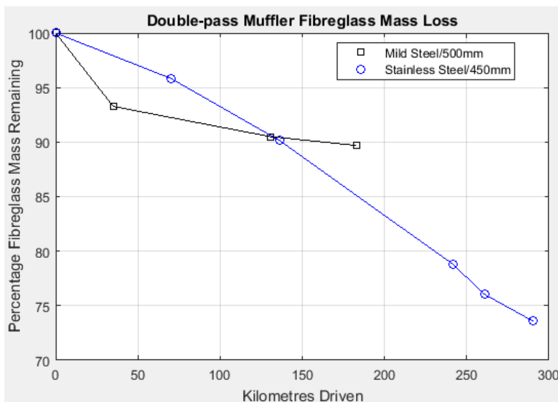
Figure 70: Fibreglass lost vs. kilometers driven. The mild steel muffler's mass seemed to almost reach a plateau before it required repacking. The stainless steel muffler, conversely, continued to lose mass at a steady rate.
