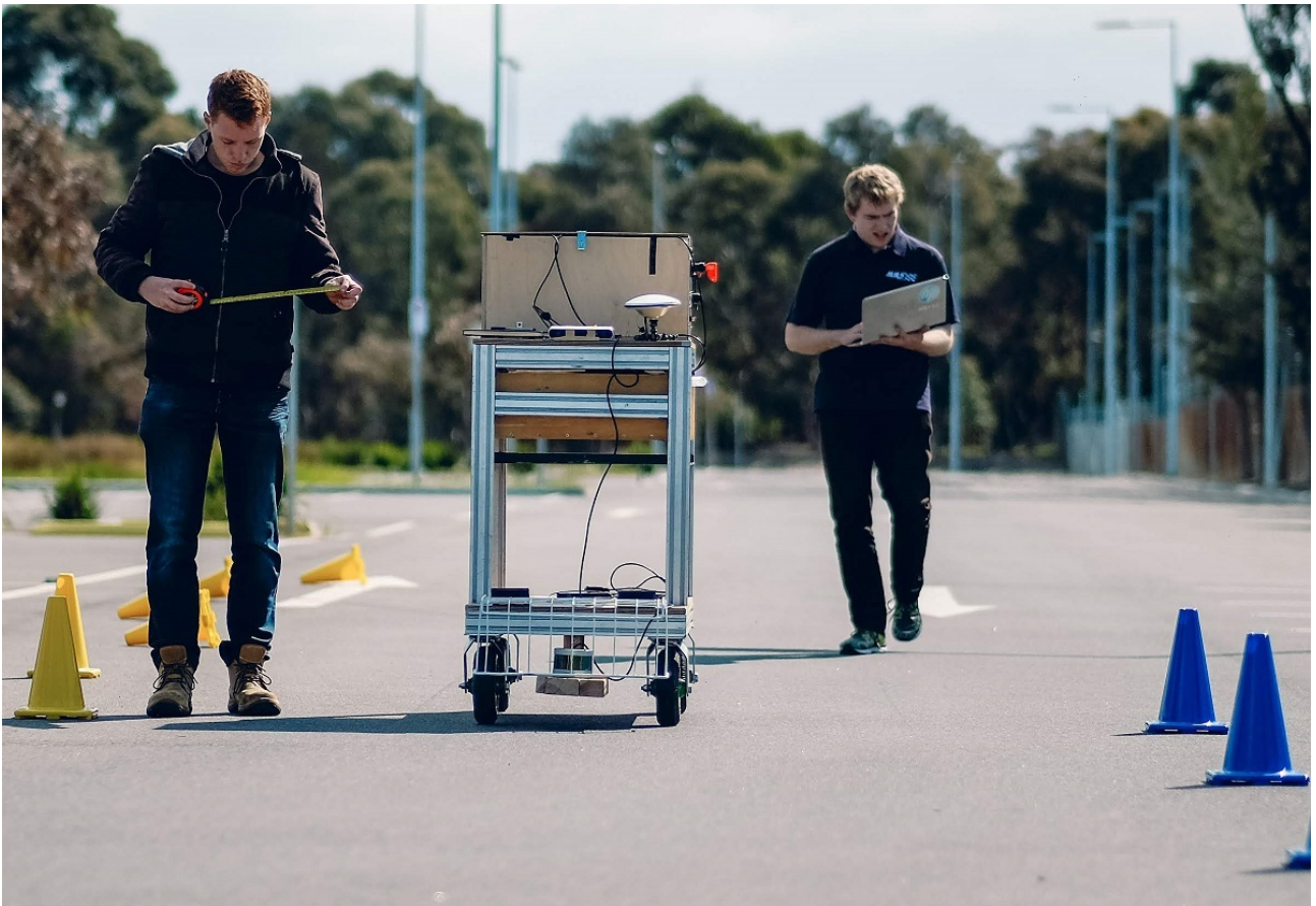
Figure 7.1: The testing trolley, recording a straight-line track marked by yellow and blue cones. Credit: Jack Coleman
