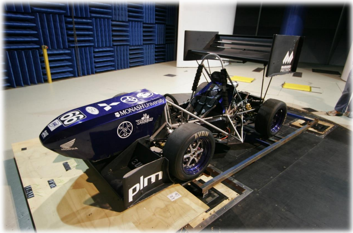
Figure ..5.2 - 2008 car setup with artificial ground plane under front wing
