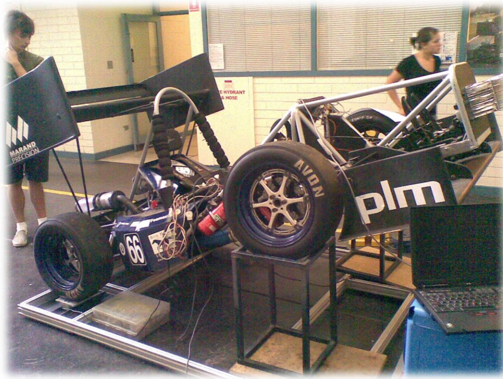
Figure ..3.2 - 2008 Vehicle with front raised on load cells.
