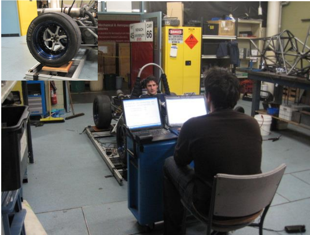
Figure ..3.3 - 2008 Vehicle on load cells with diagonal wheels shimmed
