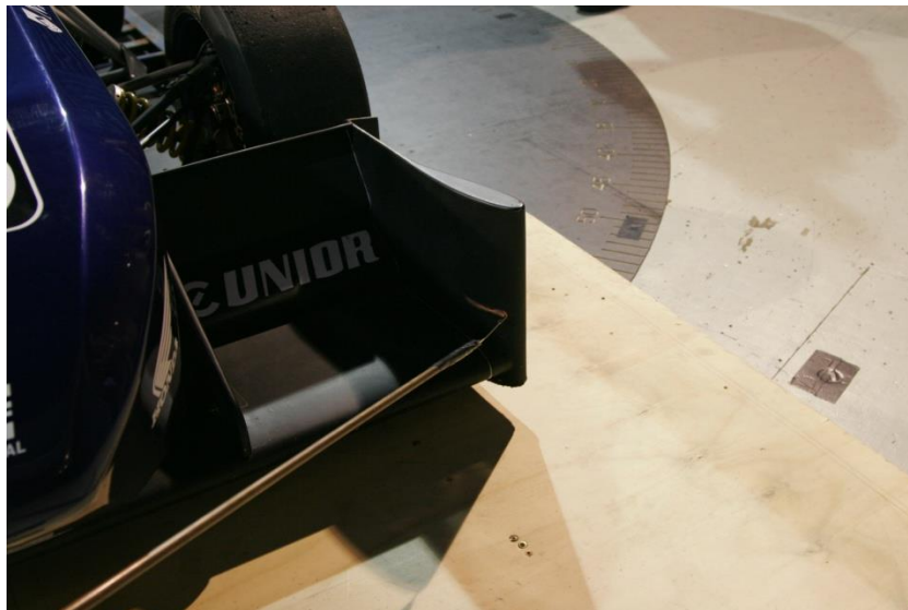
Figure ..5.11 - Initial endplate design after manufacture
