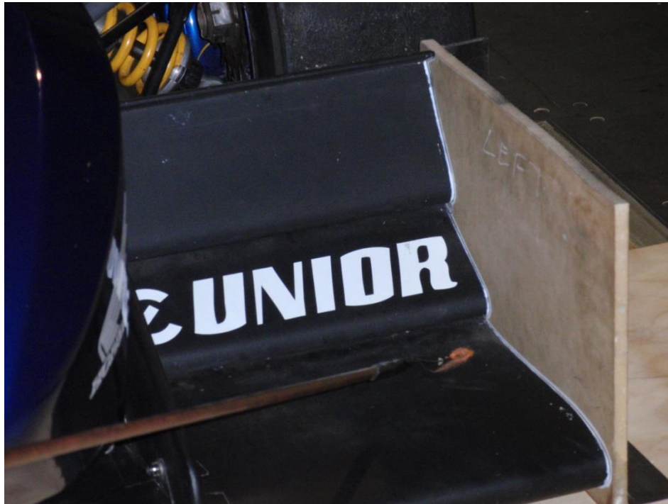
Figure ..9.2 - Front wing endplate flow visualisation, at 25° yaw. Flow visibly separates from the leading edge of the endplate causing turbulent flow over mainplane in its wake.
