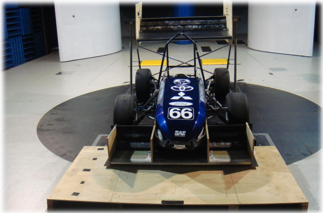
Figure ..5.18 - Full car testing of 2009 aerodynamic package with artificial ground plane
