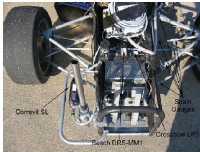
Figure ..9.5 - Correvit attached to 2003 Monash Formula SAE car
