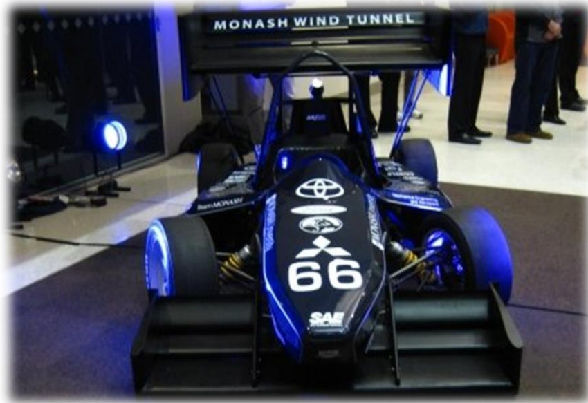
Figure ..4.7 - Fully manufactured 2009 aerodynamic package on the 2009 vehicle
