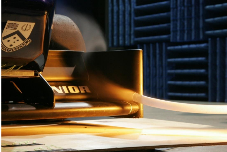
Figure ..9.3 - Front wing at 0° yaw, vortex clearly visible from smoke visualisation
