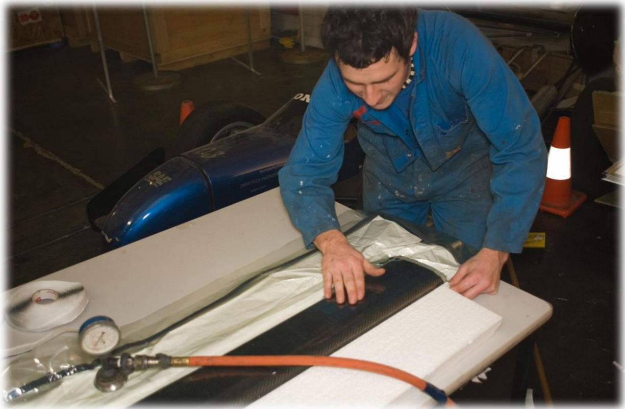
Figure ..4.1 - Flap profile being prepared for vac bag
