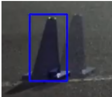
Figure 5.4: Cone skew due to rolling shutter
