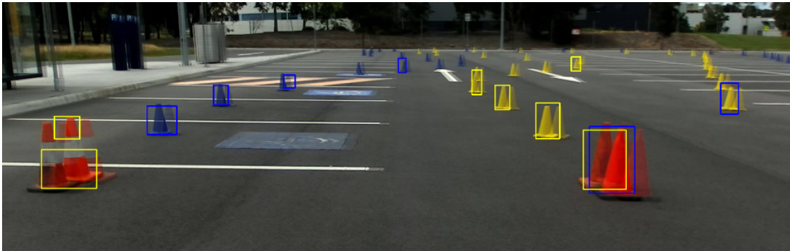
Figure 5.15: Camera cone detection output
