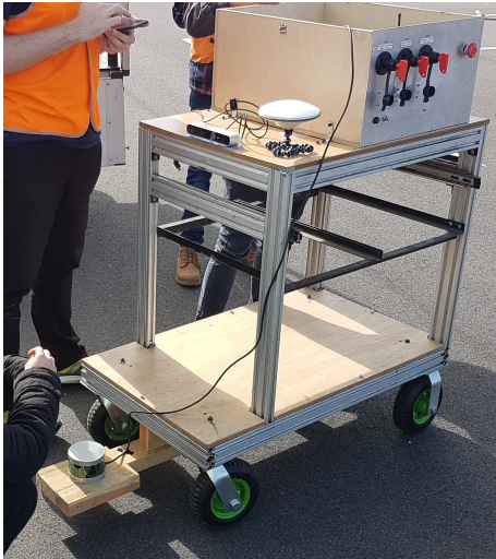
Figure 5.1: Testing trolley with mounted sensors and computing box
