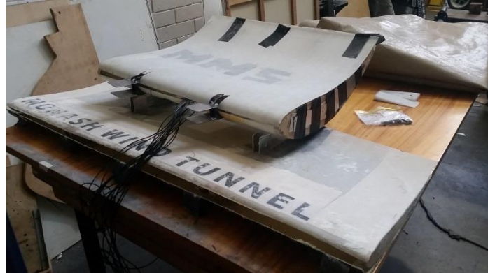
Figure 59: Rear (top) and front (bottom) mainplanes that have been pressure tapped and with all mounting attached. Requires the use of DPMS unit before testing.
