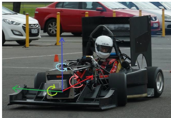
Figure 49: X (red) –Y (green) - Z (blue) and Roll (pink) –Pitch (light green)-Yaw (light blue)
