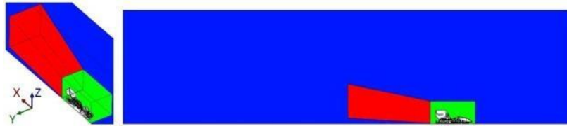
Figure 23: Fluid Domain Setup: White = Car, Green = Nearfield, Red = Wake and Blue = Farfield.
