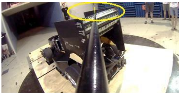
Figure 56: Tuff wand with GoPro mounted. Excellent video footage was seen from this new technique.
